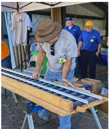
▼ Building track panels using Accu-Tie track system at the Train Mountain Triennial
