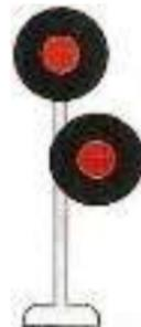
**STOP** The next switch is thrown to the diverging route which is occupied.
